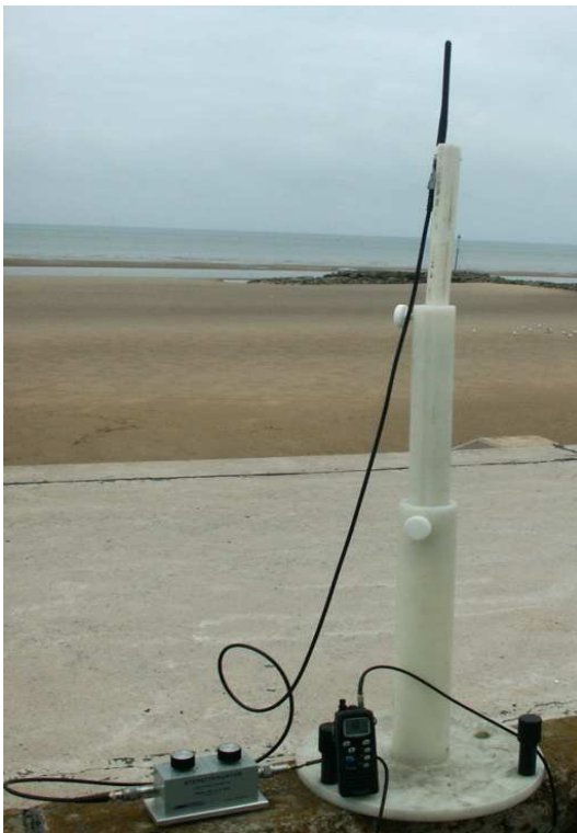
Figure 3-1: The VHF antenna and receiver set up at Prestatyn
