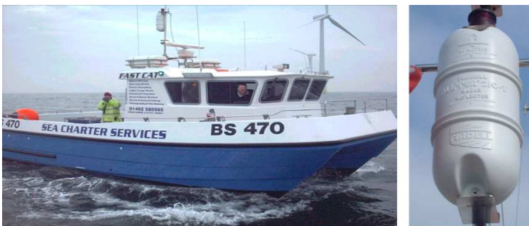
Figure 6-31: "Fast Cat" and its "Blipper" radar reflector
