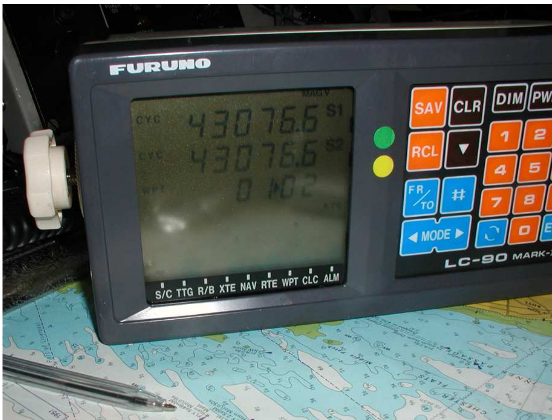
Figure 7-1: Furuno LC- 90 Loran C receiver
