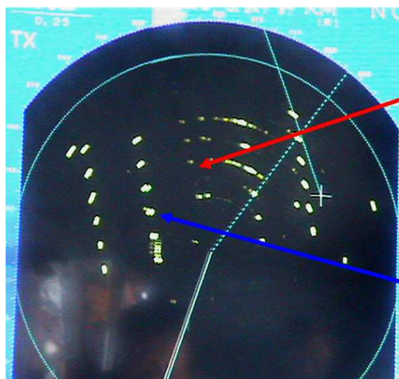
Figure 6-6: Shadow and blind arcs with side lobe echoes
